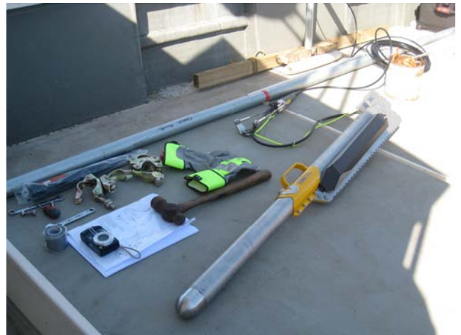
The side scan sonar equipment on the deck of the Charles-Ann prior to survey work in the Bay of Firth
