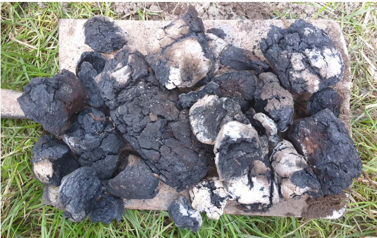
Figure 2: Some of the first batch of peat charcoal
