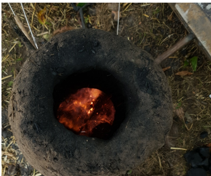
Figure 4: Fuelling one of the furnaces and getting it up to temperature
